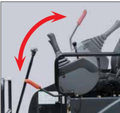
**Lock Lever Allows Lock/Neutral Engine Starting**
